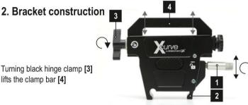
Turning "gray" clamp [1] locks/unlocks the clamping lever
